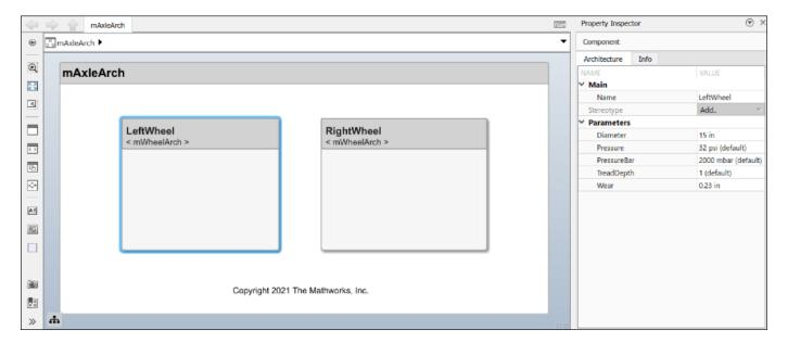
You can expose these parameters as model arguments and then edit the parameters as instance-specific parameters independently for each component that references the same model. Right-click the RightWheel component and select Block Parameters (Model Reference). Click the Instance parameters tab and select the Argument check box for the new parameters Pressure and TreadDepth.
