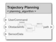
Any change made in an architecture model reference is immediately reflected in the models that link to it. If you move or rename the referenced architecture, the link becomes invalid and the linked component displays an error. Link the component to a valid architecture model reference.
